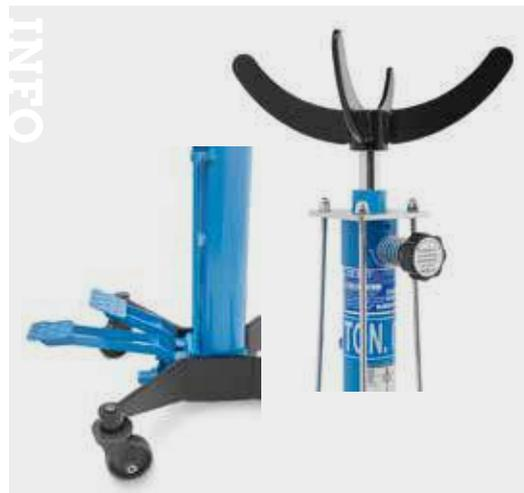
**CRIC HYDRAULIQUE POUR TRANSMISSION OMCN D'UNE CAPACITÉ DE 1000 -1500KG.**
